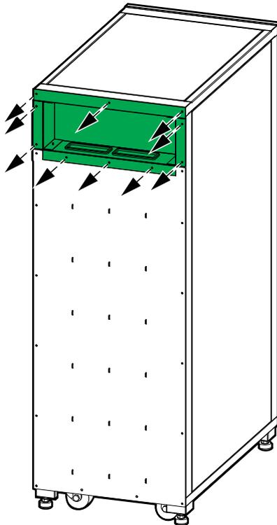
2. Rotate the conduit box and install.
