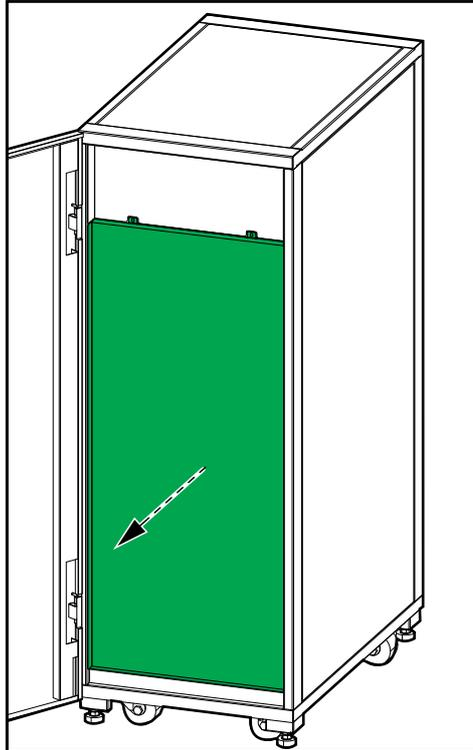
2. Holding the handle, install the battery modules one string at a time from the bottom and up.
