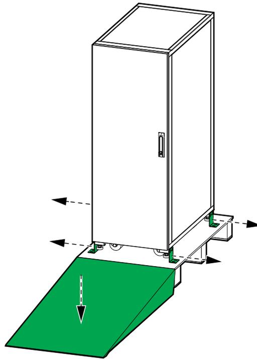
4. Loosen the bolts and remove the shipping brackets. Dispose of the shipping brackets.
