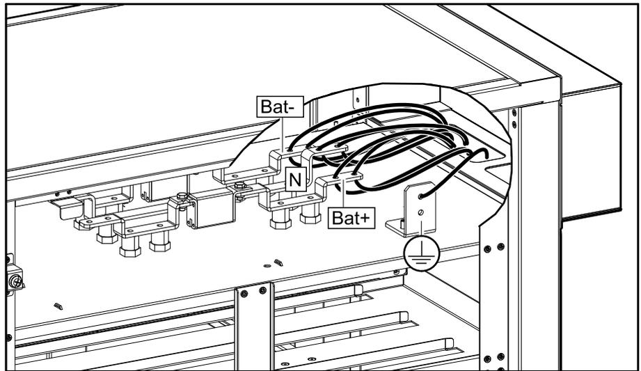
5. If more than one modular battery cabinet is part of the installation, connect the battery cables (kit E3MOPT006) between the modular battery cabinets.
