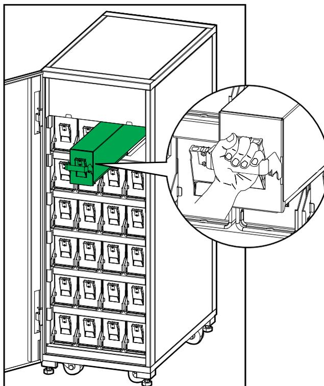
3. Push down the handle of each battery module and fasten with the provided screw in front of the battery module.
