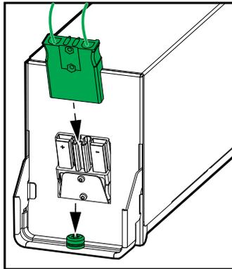
4. Remove the shrink tubes from the power terminals and connect the power terminals to the batteries.
